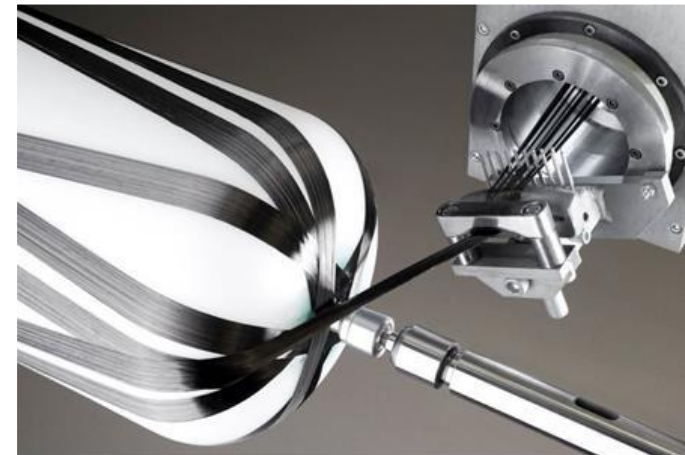
Winding of carbon fibres onto HDPE liner
