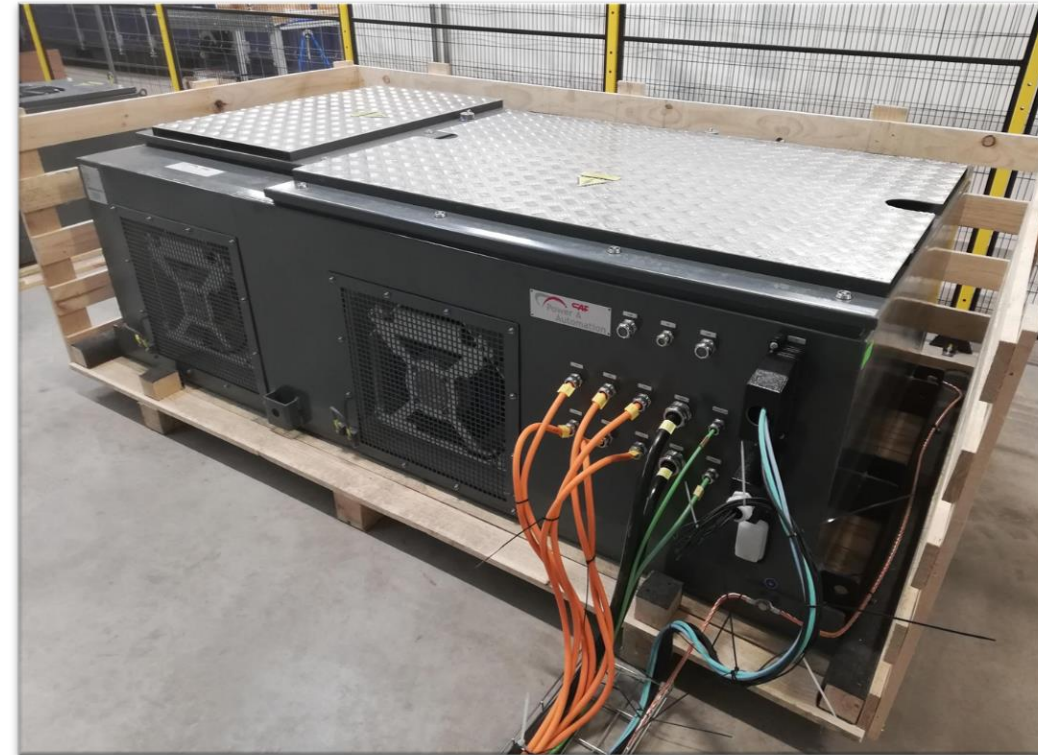
Energy storage with BTMS and DC/DC placing, mechanical and electrical installation
